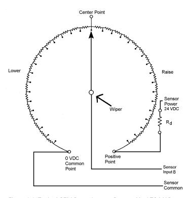
Figure 3-8: Typical OEM Potentiometer Powered by LTC-MAP To calculate  $R_{\mbox{\scriptsize d}} \colon$
